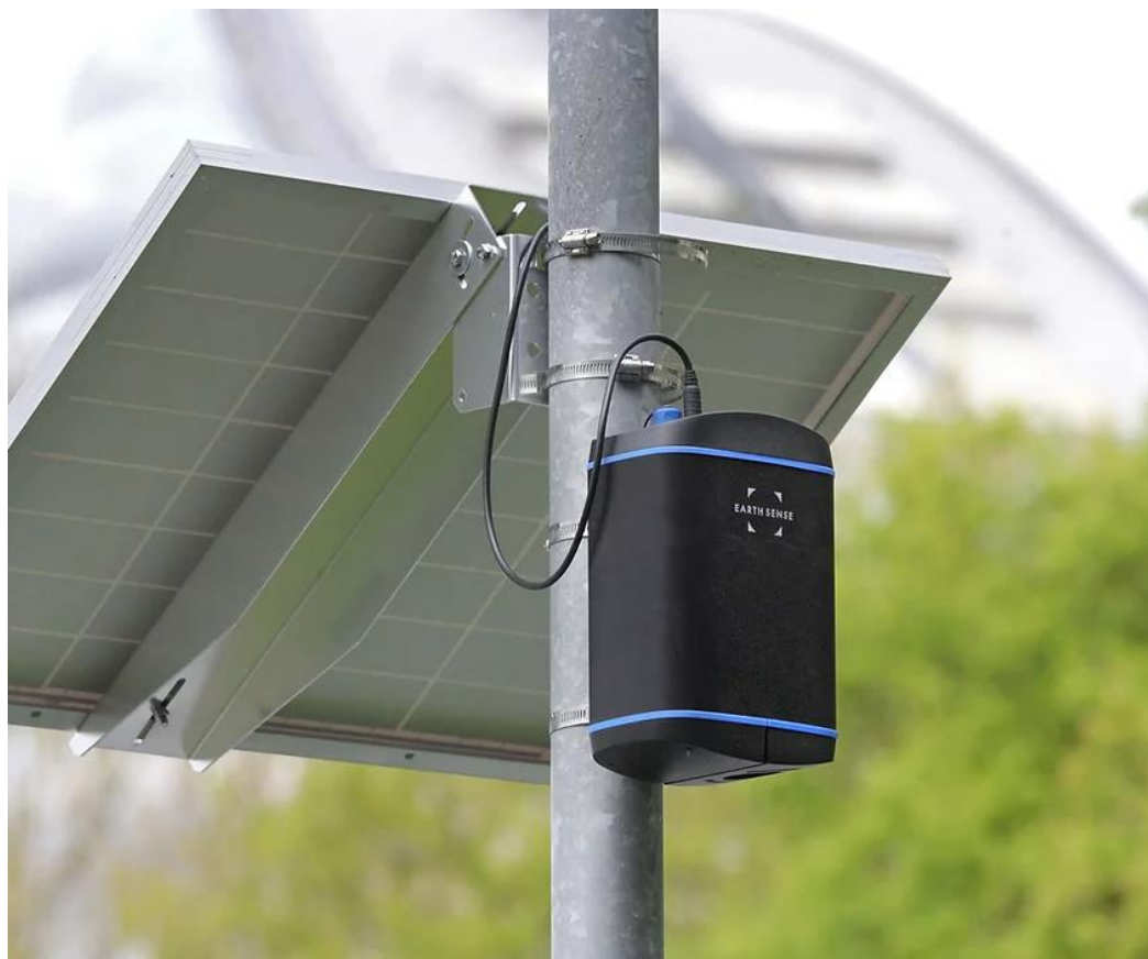
Figure 2. Typical Earthsense Zephyr Installation
